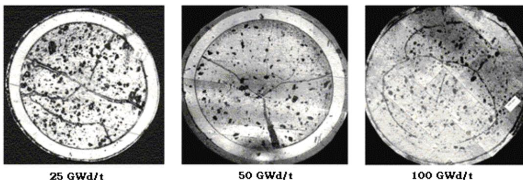
*FIG. 3. Photomicrographs of Mark-I Carbide Fuel at Various Burn-up Levels*
