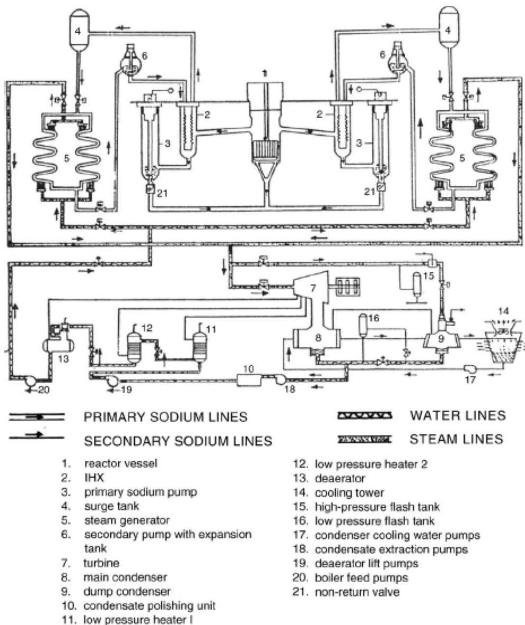
FIG. 1. Flow-sheet of FBTR.
