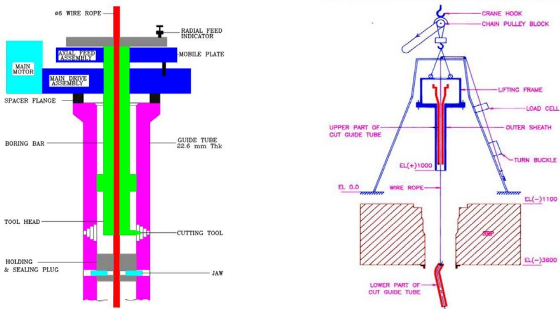
FIG. 5. Guide Tube Cutting and Retrieval
