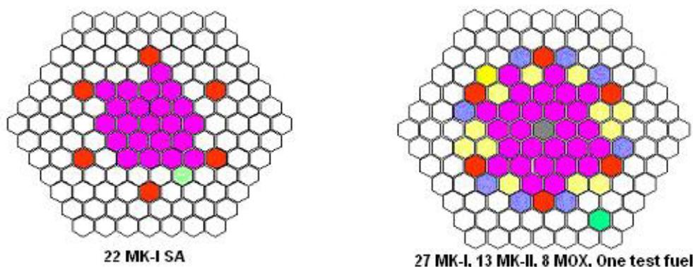
FIG. 2. Core configuration at first criticality and as of now
